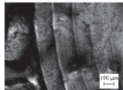
Figure 16. Topography of a paint print on polyester film after the ball-on-disk test, after 30min under a load of 2N.
